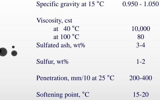
Residue contains high quantity of polymers and metals and can be used for asphalt blending, production of paving asphalt, bitumen protective covering or as fuel in the cement factories.
